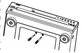
If the shipping screws are still in place and the power is turned on, the disc tray will not open. If this happens, turn off the power, unplug the power supply cord from the power outlet and remove the shipping screws. Retain these screws as they will be needed when the player is transported.
