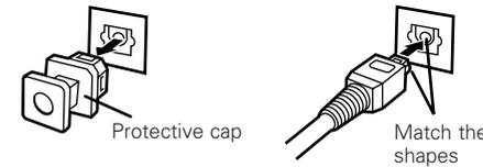
Remove the protective cap, match the shapes then insert firmly all the way in.
