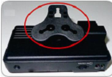
**2.** Assemble the sucking disc and Micro SD card.
