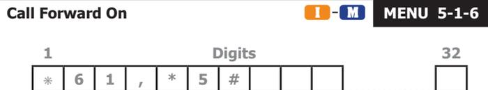
The panel is able to activate certain Telco services such as Call Forwarding when the system is armed. Call forwarding means that your customer will no longer need to remember to manually activate the Call Forward On feature via the telephone before leaving.
