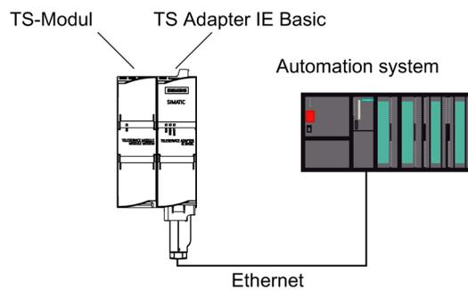
Figure 3-6 TSA IE Basic direct connection to the automation system S7
