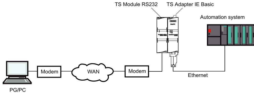
Figure 1-6 Connection to an external modem
