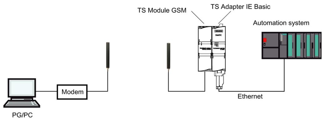
Figure 1-5 Connection to the GSM network
