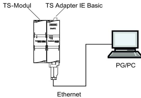
Figure 3-5 TSA IE Basic direct connection to PG/PC
