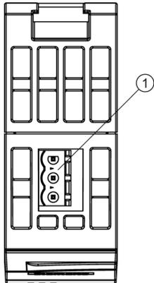
① Power socket for the 24 V DC Power Supply
