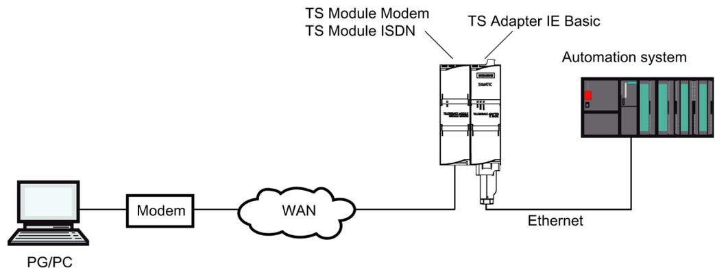
Figure 1-4 Direct connection to the telephone network
