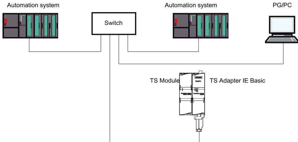
Figure 3-7 Direct connection in a networked system
