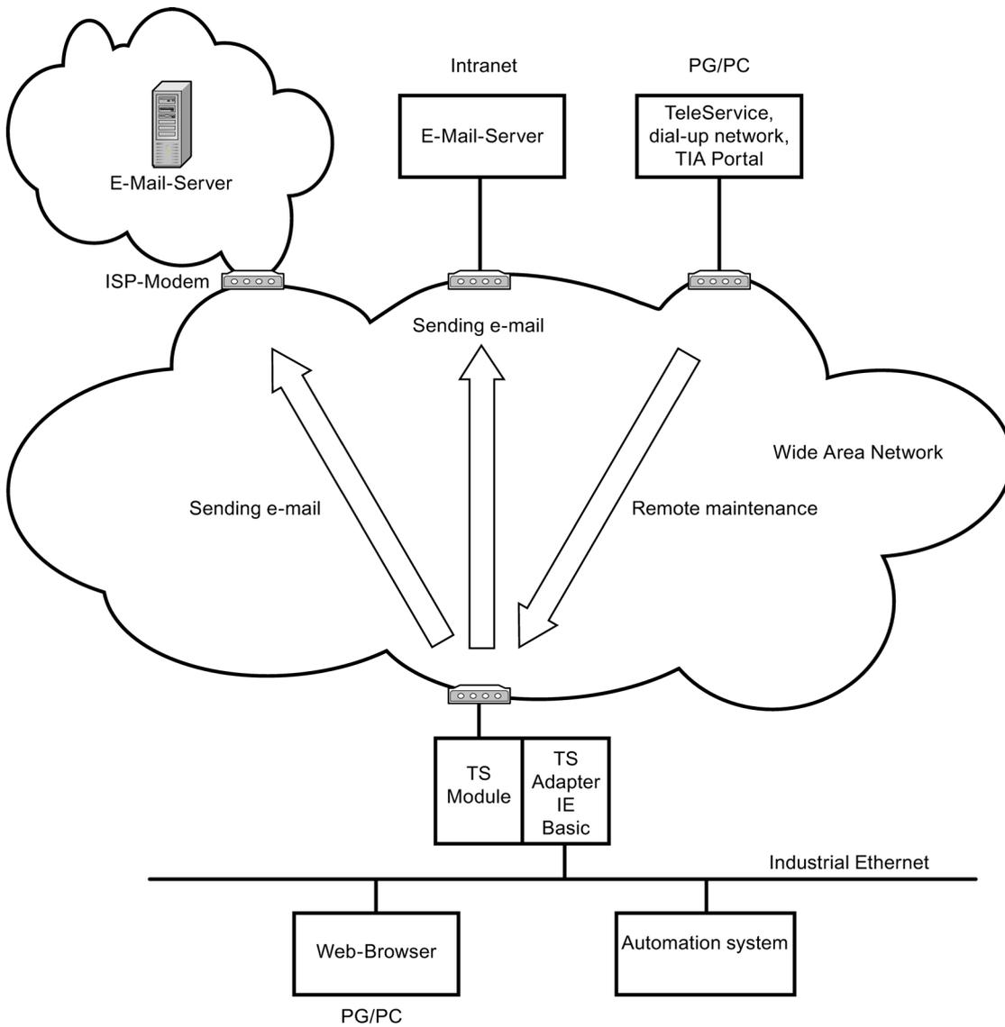
Figure 1-2 Functions of the TS Adapter IE Basic
