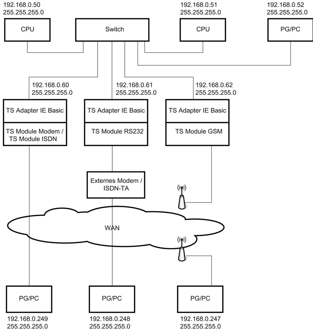
Figure 4-1 Example of a networked system
