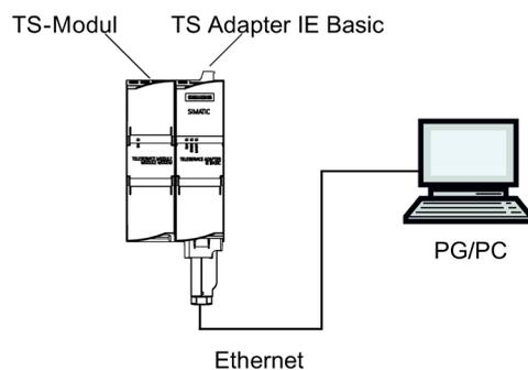
Figure 1-3 Direct connection
