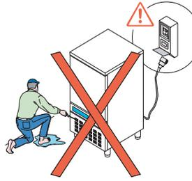
do not touch the appliance if hands and/or feet are wet. Before performing any cleaning or maintenance disconnect the appliance from the electrical source and carefully unplug the appliance. Do not remove safety guards. Wear protective gloves when cleaning the condenser. Do not use scissors, screwdrivers and sharp objects on the cooling circuit.
