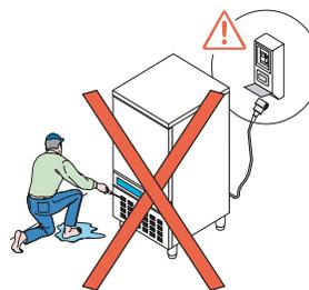
**do not touch the appliance if hands and/or feet are wet. Before performing any cleaning or maintenance disconnect the appliance from the electrical source and carefully unplug the appliance. It is DANGEROUS AND UNADVISEABLE to remove the safety guards, AND IS NOT REQUIRED for routine maintenance. Wear protective gloves when cleaning the condenser. Do not use scissors, screwdrivers and sharp objects on the cooling circuit.**
