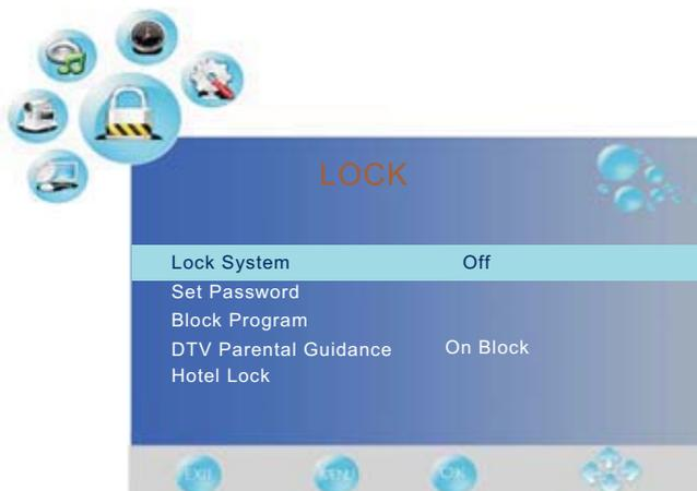
Use the ◀ and ▶ buttons to select the **LOCK** menu(as the picture above), press ▼ button to enter the menu.
