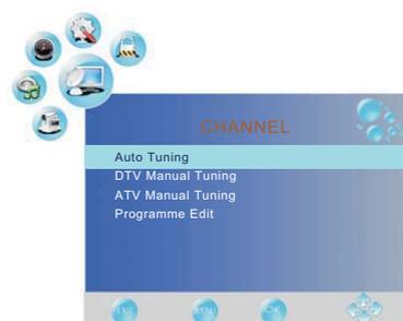
3. Use the ▼ / ▲ buttons to select an option of the sub-menu, and press the ▶ button. While in adjustment mode, use the ◀ / ▶ button to change the value of the item.
