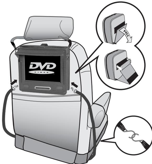
6. Secure the Travel Theater to your seat by adjusting the straps to the appropriate length.
