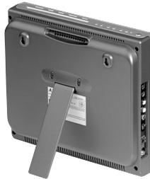
3. Connect the supplied AC adapter's barrel plug to the Travel Theater's **DC 12V** jack.
