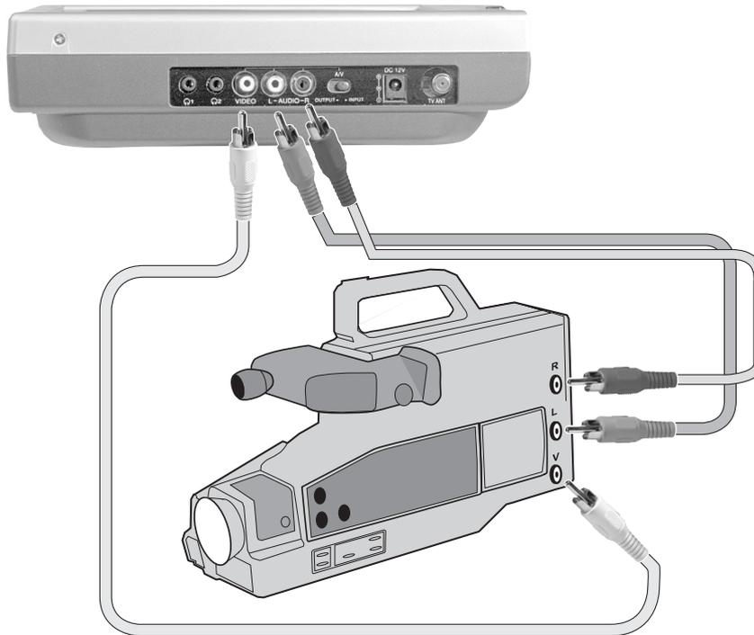
1. Connect the audio/video cable's white plug to your device's left output socket. Connect the other end of the cable to the Travel Theater's **AUDIO L** jack.
