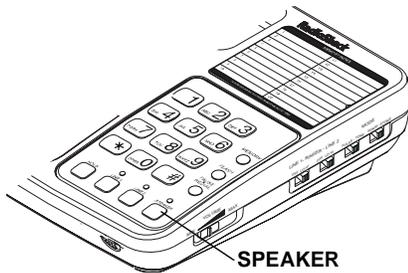
When you receive a call, that line's indicator flashes. To answer the call, press the line button (**LINE 1** or **LINE 2**) below the flashing indicator and lift the handset or press **SPEAKER**.
