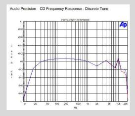
Using the analog outputs of the Apex player, and no P-1A or P-3A, the frequency response is terrible.
