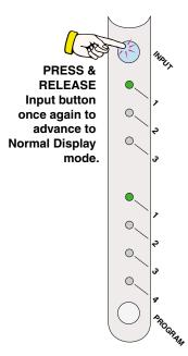
When you press the Input button the display will return to Normal with green LEDs indicating the active Input and Program selections.
