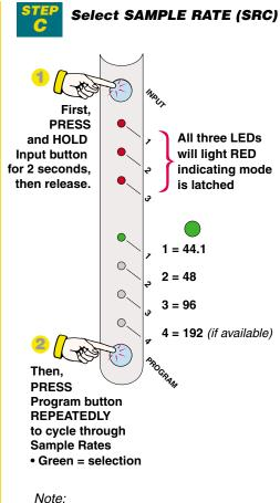
• Each of the 3 Inputs has its own Sample Rate setting.
