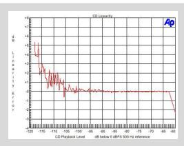
The P-3A, when using the digital output of the Apex, shows DAC linearity easily to the -96 dB limit of 16 bits, and actually remains linear below that limit, although the graph eventually rises due to the content added by the noise floor caused by the desirable presence of dither, which allows encoding greater than 16 bit resolution onto a 16 bit system at the expense of a higher theoretical noise level than, say, a 20 or 24 bit system.
