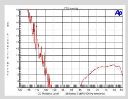
To be fair, the plot here is offset by roughly -0.7 dB, but you can still see that even after adjusting the plot to match 0 dB with where the chart starts recording (at about -62 dB), the DACs on the Apex only remain linear to about -75 dB, falling far short of the resolution capable with even standard CD sources, akin to the medium of the vinyl LP. The plot falls absolutely off the chart between -100 dB and - 105 dB, and only rises back due to the noise floor.
