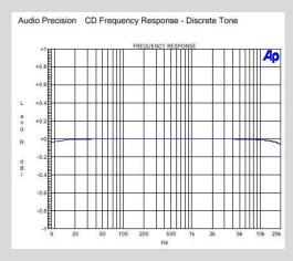
Notice how the frequency response stays close to 0 dB throughout the audible range. Red and blue lines in the graphs represent left and right channels.
