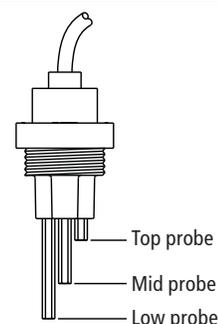
Tank-level icons indicate water level at the water level control probe. See "Water level control" on Page 55.
