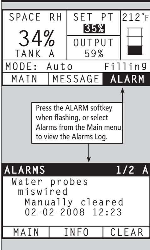
The Alarms menu displays system alarms. Using the keypad/display, go to the Alarms menu by pressing the Alarms softkey (which will be flashing if there is an Alarm), or by pressing the Home softkey and then the Alarms softkey. Using the Web interface, click on the View Alarms link in the upper left corner of any screen.
