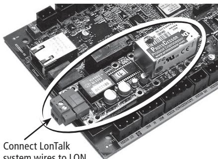
Connect LonTalk system wires to LON ProtoCessor module here.
