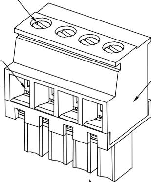
Terminal block plug. Make connections when the plug is attached to the board, or remove for easier access. Pull plug straight up to remove.
