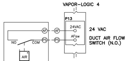
DUCT AIR FLOW SWITCH IS IN SDU CABINET
