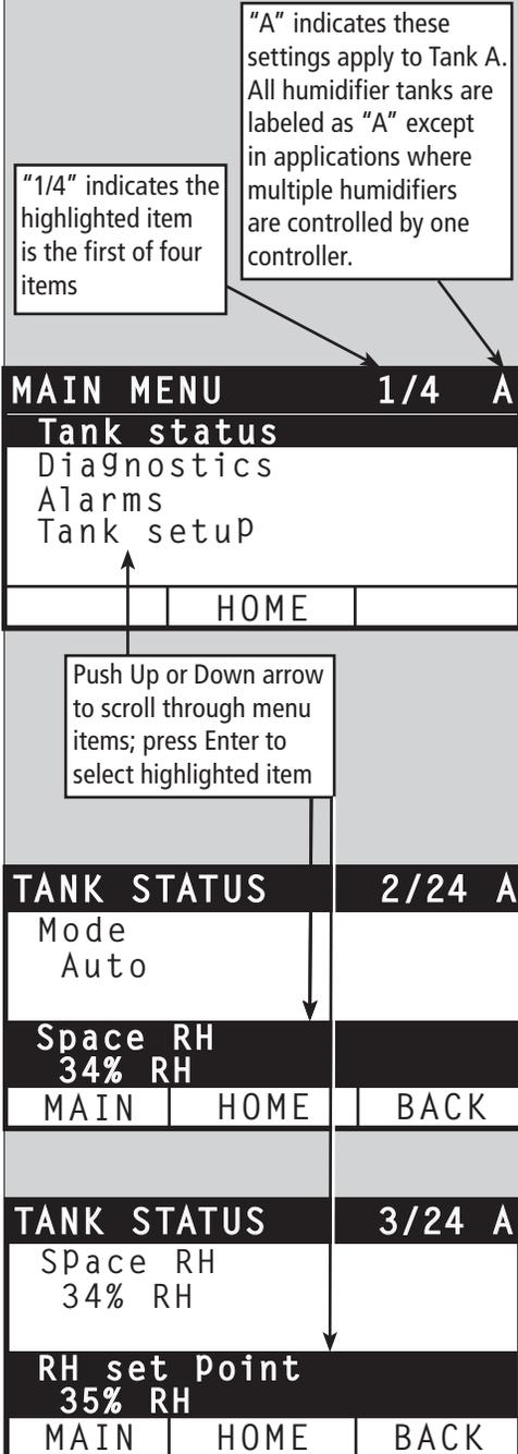
Using either the keypad/display or the Web interface, the Status screen is where all humidifier parameters can be viewed.
