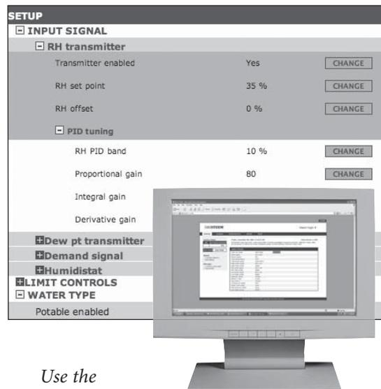
*Use the Vapor-logic4 keypad/display or the standard Web interface, shown here, to control your humidification system.*
