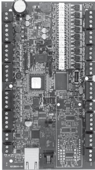
Terminals P-11 through P-16 have a white border on the Vapor-logic4 board. This is where you will make most of your field wiring connections.
