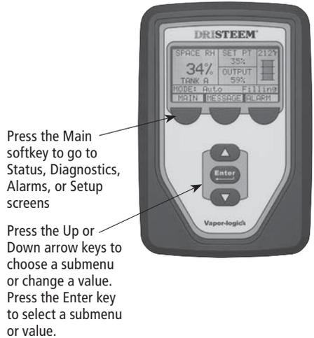
Vapor-logic4 keypad/display has the following menus and screens:
