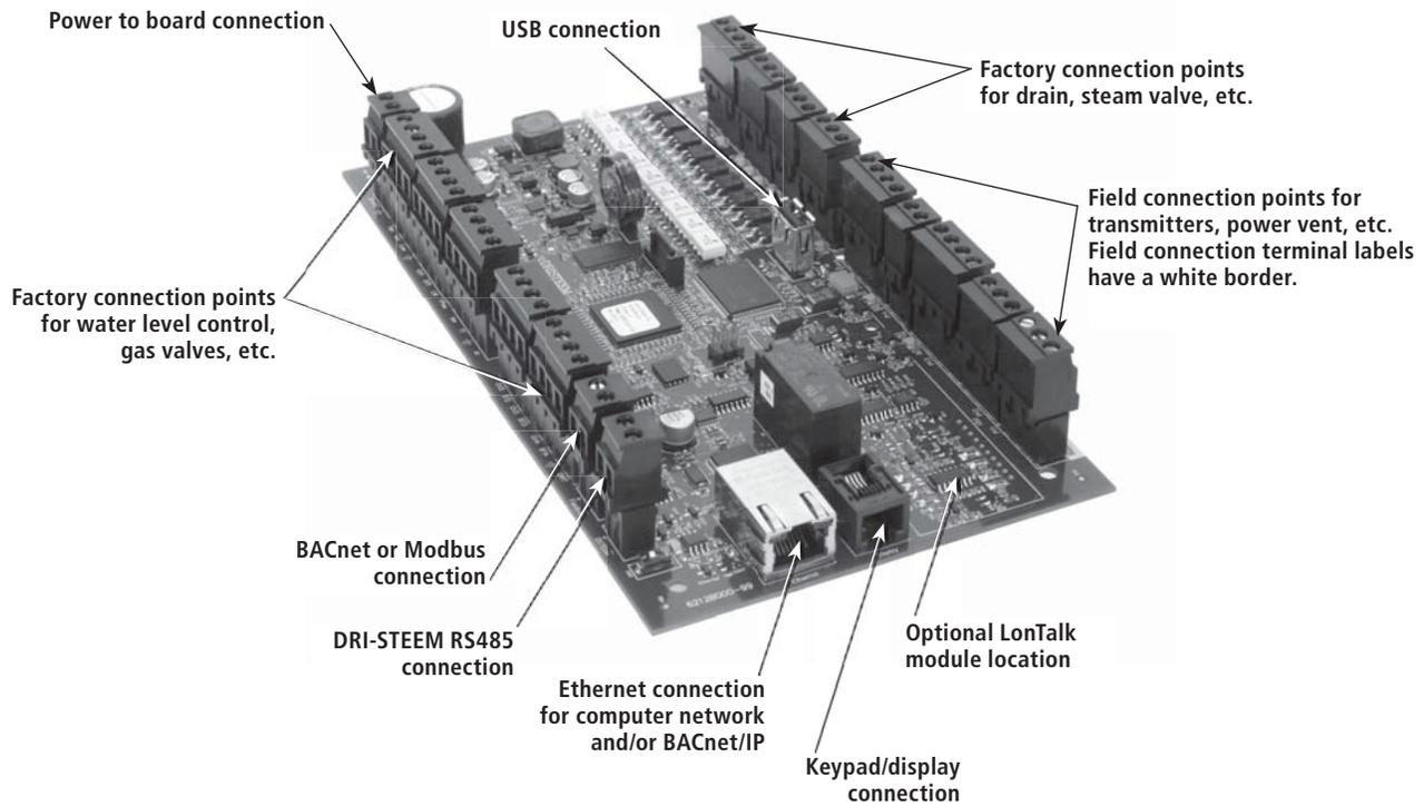
The photo above shows key components of the Vapor-logic4 control board. See the illustration on the next page for more detail.
