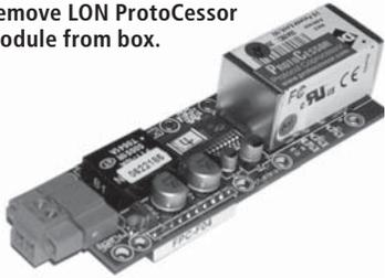
2. Insert LON ProtoCessor module into pins on Vapor-logic4 board.
