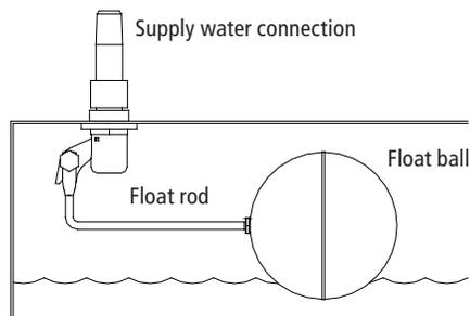
Humidifiers using DI/RO water control water levels using a float valve and low-water cutoff switch.
