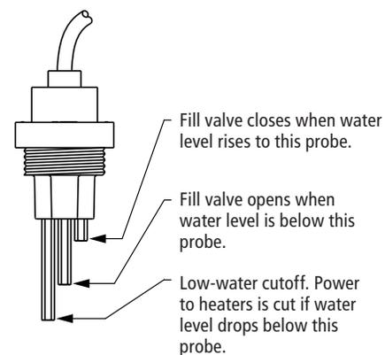
Humidifiers using tap or softened water control water levels electronically using a three-rod probe. The controller responds with the above actions when the water level reaches each rod.
