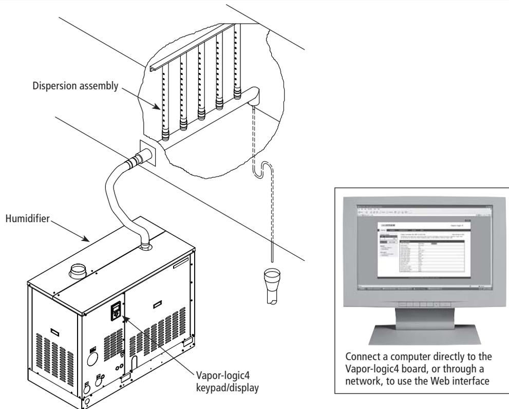
Every humidification system with a Vapor-logic4 controller has a keypad/display connection and an Ethernet connection for connecting to a Web interface on a computer. A GTS humidifier is shown here, with keypad/display mounted on the cabinet. Other types of DRI-STEEM humidifiers can have the keypad/display contained within a control cabinet or mounted remotely.
