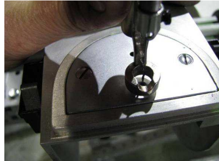
Figure 3.23 – Press on the needle bar gently to center needle in hole
