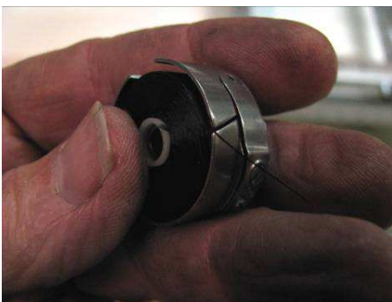
Pull the release Latch and remove the bobbin case
