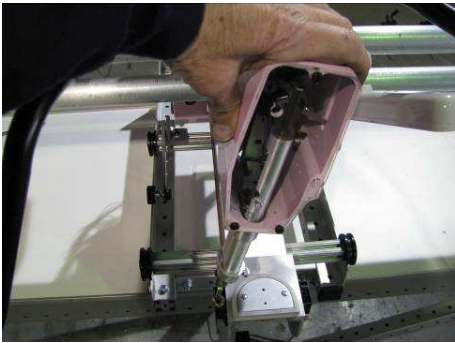
Figure 3.21 – Continue holding lever and rotate until the head locks
