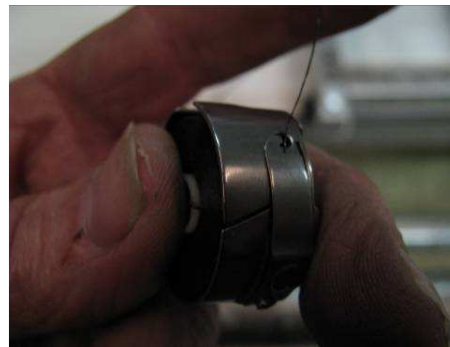
Pull the release Latch and remove the bobbin case
