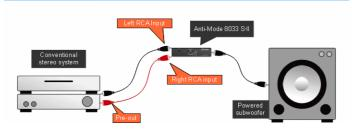
The dual line inputs of Anti-Mode 8033S-II are used when connecting into a 2.1 stereo system which has only stereo preouts available (no dedicated LFE or sub output).
