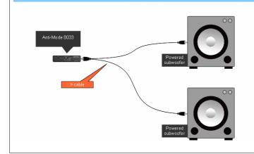
Two or more subwoofers can be connected using a splitter Y-cable, or by using the inverted-phase output of the 8033S-II and inverting phase on the subs connected to it.
