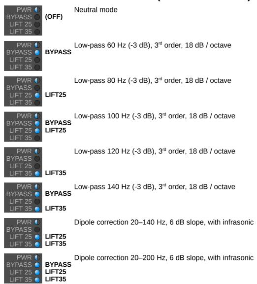
If you are going to use the dipole modes with your subwoofer, activate and save the filter setting before Anti-Mode calibration. The dipole correction filters are active during calibration to correct the open-baffle subwoofer's natural attenuation of bass in the lower frequencies. Other modes do not affect calibration and can be activated and deactivated at any time.
