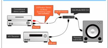
The dual line inputs of the Anti-Mode 8033S-II also allows you to connect both a home theater and stereo system at the same time. An additional stereo-to-mono converter cable is required.
