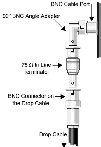
**Note:** The 90° BNC angle connector is not available from Modicon. See *RIO Cable Material Suppliers*, p. 143 for a list of suppliers.
