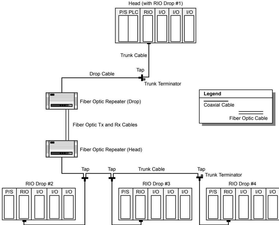
The distance between the two repeaters is limited by the maximum allowable attenuation of the fiber optic cable used in the installation. Fiber attenuation is calculated separately from coaxial cable attenuation (see *Attenuation Considerations in an Optical Path*, p. 56 for more details).
