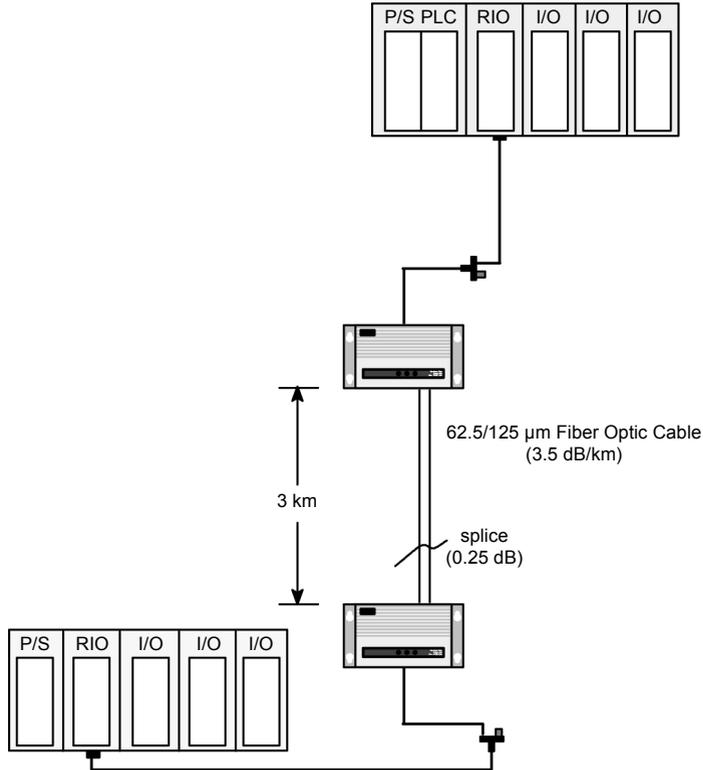
The specified power loss budget for a link using this optical cable is 11 dB. We know that the cable's attenuation over 3 km is  $3.5 \text{ dB/km} \times 3 = 10.5 \text{ dB}$ , and we are given an attenuation of 0.25 dB for the cable splice. Thus, we have a total optical power loss of 10.75 dB on the link, which is under budget and therefore legal.
