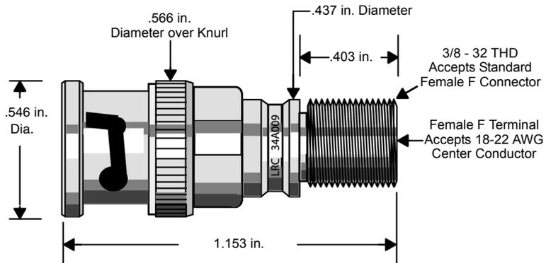
The 52-0614-000 Adapter permits the F connector on an RG-11 trunk cable to be attached to the BNC connector on an RIO processor at the network head-end or the F connector on an RG-11 drop cable to be connected to a J810/J812 or J890/J892 drop adapter at the drop.
