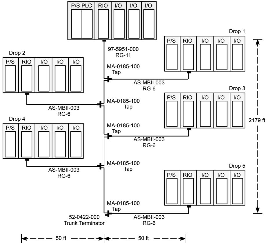
This system uses RG-11 cable for the trunk; for illustration purposes, its specified attenuation is 0.24 dB/100 ft at 1.544 MHz. Running to the adapter at drop 5 is a Modicon AS-MBII-003 RG-6 drop cable, a 50 ft cable with an attenuation of 0.3 dB. To calculate end-to-end attenuation on the trunk cable (TCA), multiply 0.24 dB (the trunk attenuation per 100 ft) by 21.79:
