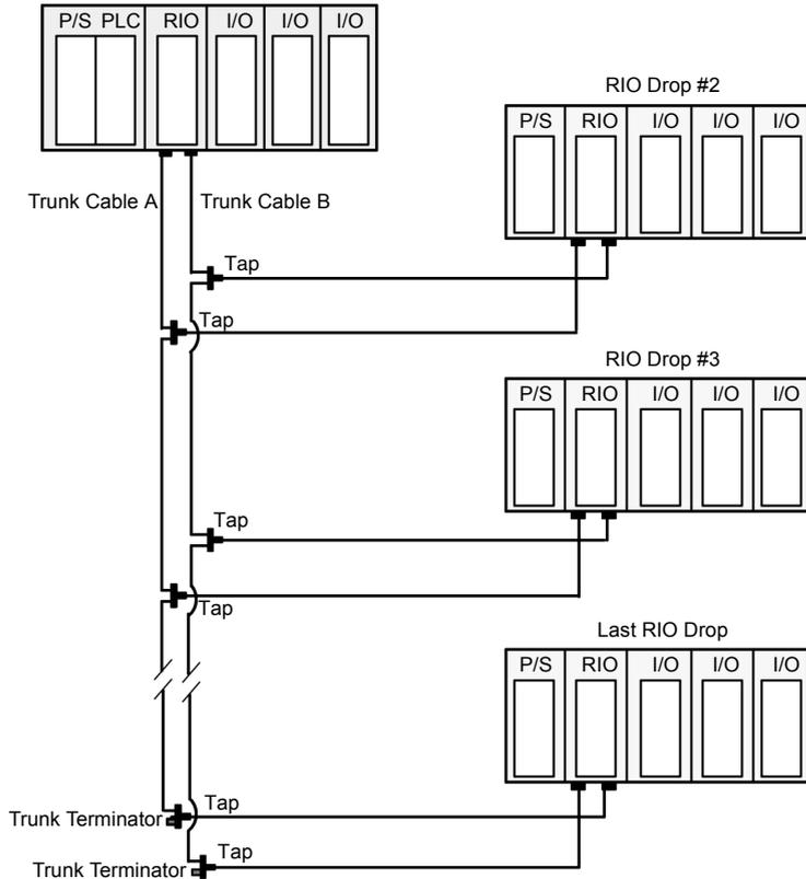
The two cables are treated as two separate networks, and each cable is an independent system running from the same RIO processor node to the same remote I/O drops. If a break occurs in cable A or cable B, an LED goes ON at the RIO head processor. The condition is also logged in words 179 ... 277 of the status table: these status words can be accessed via the STAT instruction (see *Modicon Ladder Logic Block Library User Guide*, 840 USE 101 00).
