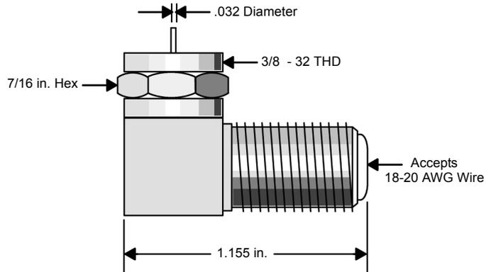
Modicon has also approved the FF90FM right-angle F adapter manufactured by LRC Electronics and the GFMF/90 right-angle F adapter manufactured by Gilbert Engineering. See *RIO Cable Material Suppliers*, p. 143 for contact information.
