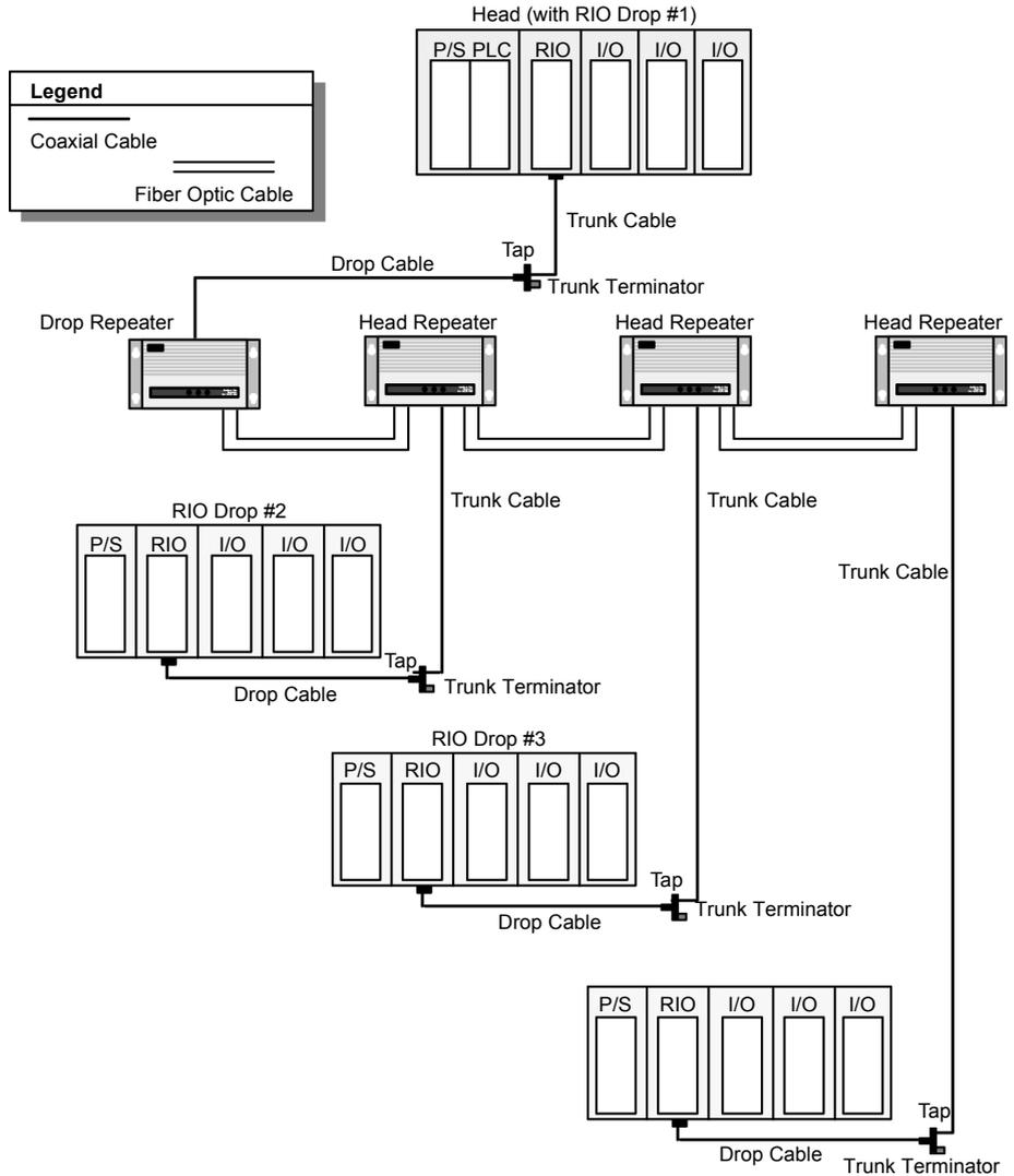
Five chained repeaters can be linked in a bus topology. This number can be reduced by the total pulse width distortion (jitter) that occurs on the system.
