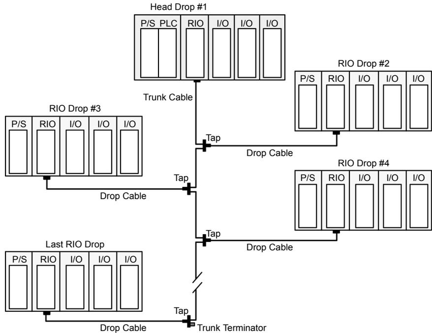
**Note:** Because this example uses local I/O at the head, the first remote drop in the network is I/O mapped as drop #2. If the PLC you are using does not support local I/O—e.g., the 984A/B PLCs—then the first drop in the RIO network can be mapped as drop #1.
