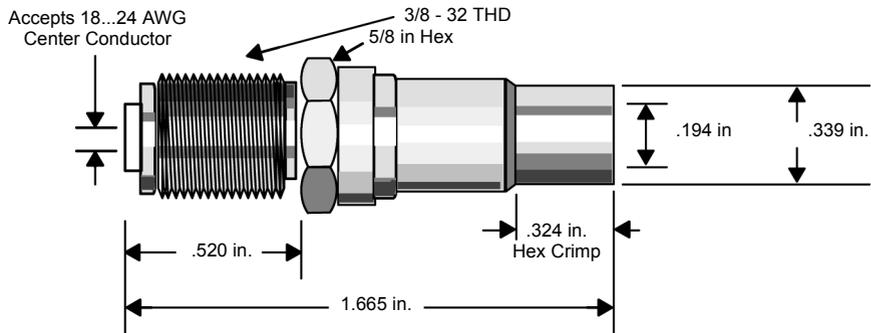
Both of these self-terminating F adapters have a return loss of 22 dB, a frequency range from 100 kHz ... 30 MHz, and an insertion loss of 0.03 dB.
