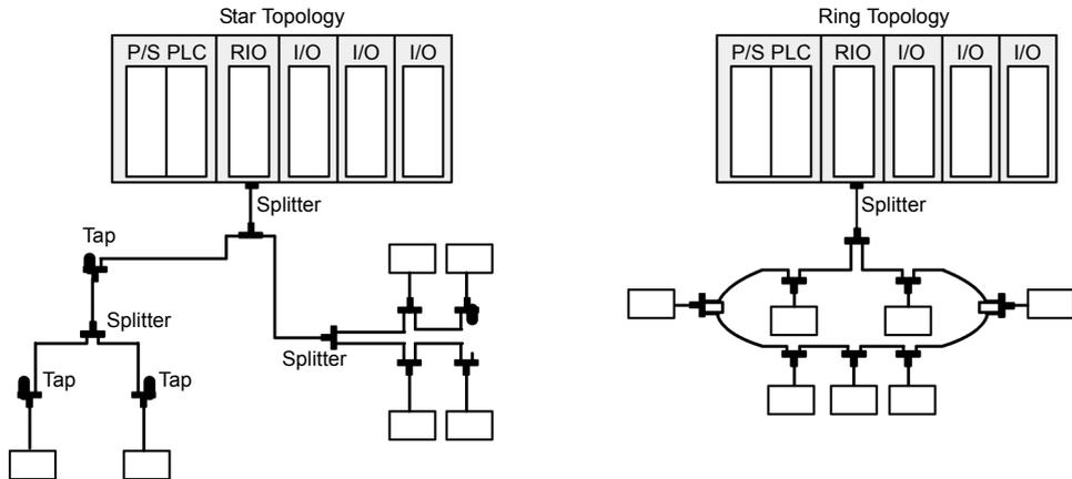
**Note:** These kinds of topologies are also not permissible when fiber optic cable is used. See *Using Fiber Optics in an RIO System*, p. 34.
