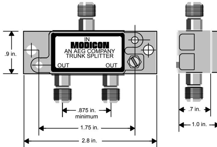
**Note:** When not in use, splitter ports must be terminated with a Modicon 52-0402-000 Port Terminator.
