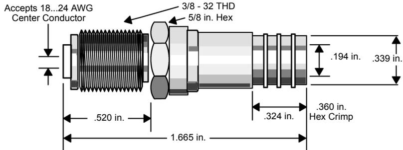
A Modicon 52-0399-000 model for non-quad shield cable
