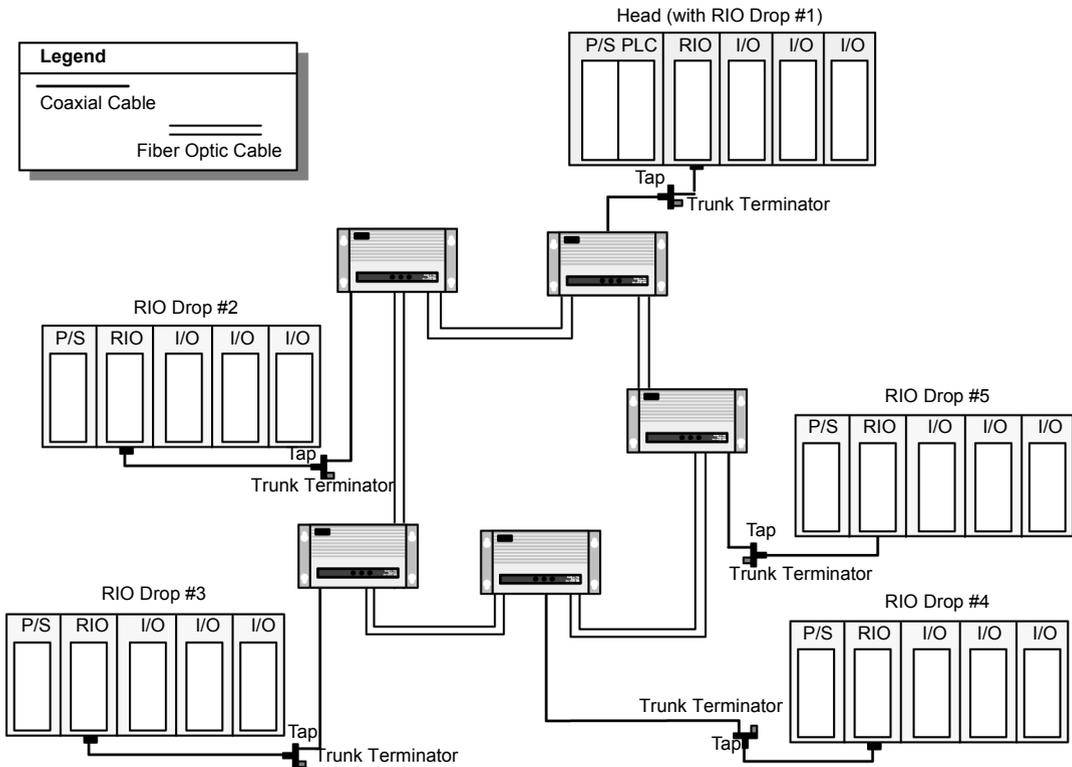
The RIO signal is sent down both legs of the ring by the drop repeater—simultaneously to the head repeaters. A feature is built into the repeaters so that when a signal is received on one of the Rx lines the other Rx channel is blanked—this prevents the same signal from being transmitted twice in the ring.
