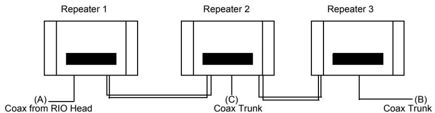
in the diagram above, jitter contribution is 50 ns from point A to point B. The following represents individual jitter contributions as shown in the diagram:
