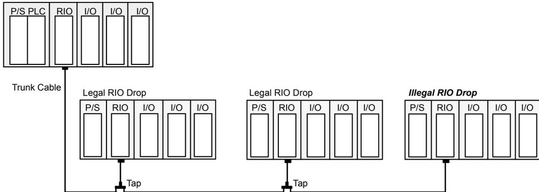
All remote drops on an RIO network must be connected to a trunk cable via a tap and a drop cable, and the last tap on a trunk cable must be terminated with a 75  $\Omega$  Modicon 52-0422-000 Trunk Terminator.
