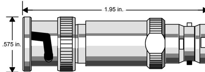
The 60-0513-000 In-line Terminator has two BNC connectors—a female for the incoming drop cable and a male to connect to the drop adapter. It has a return loss of 20 dB (VSWR 1.2:1), a frequency range from DC ... 300 MHz, and an insertion loss of 0.03 dB.
