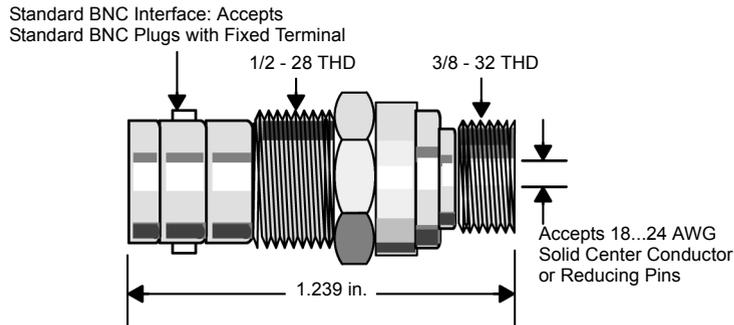
The 52-0370-000 Self-terminating BNC Adapter has a return loss of 40 dB, a frequency range from 100 kHz ... 30 MHz, and an insertion loss of 0.03 dB.
