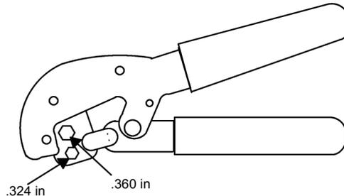
The Modicon 043509432 Crimp Tool is used to install BNC connectors onto RG-6 cable. The tool makes two sizes of hex crimp: 0.276 in. and 0.325 in. Consult Sales, available by special order only.
