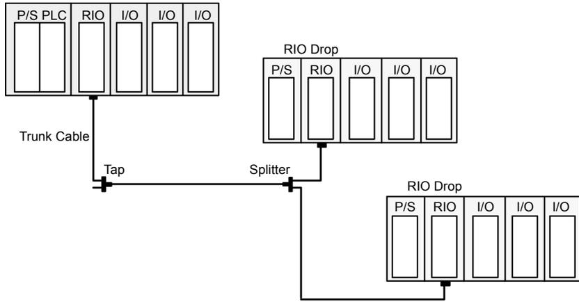
**Note:** Branching is permissible when fiber optic cable is used. See *Using Fiber Optics in an RIO System*, p. 34.
