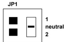
It is shipped in the neutral position—i.e., with the switch midway between position 1 and 2. The jumper can be placed in either the 1 or 2 position if the repeater is being configured as a head repeater on the optical link such that:
