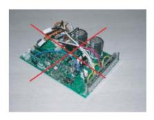
Do NOT lay the circuit board assembly flat.
