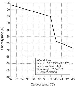
\* Capacity ratio: 100% = 5.2 kW
