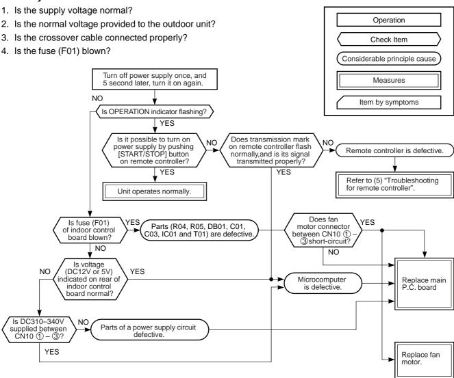
Be sure to disconnect the motor connector CN10 after shut off the power supply, or it will be a cause of damage of the motor.
