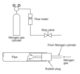
Fig. 3-5-1 Prevention of oxidation during brazing
