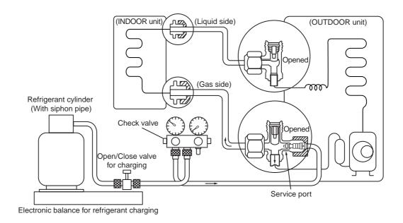
Fig. 3-4-1 Configuration of refrigerant charging
