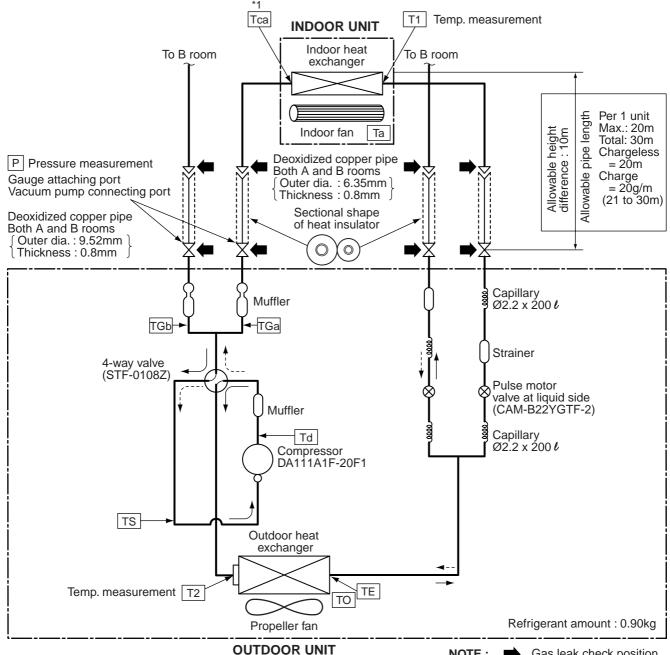
\*1 The TC sensor is at the center of the indoor unit's heat exchanger.
