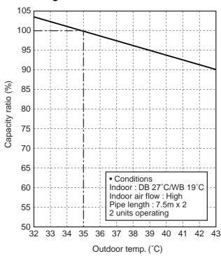
\* Capacity ratio: 100% = 4.0 kW
