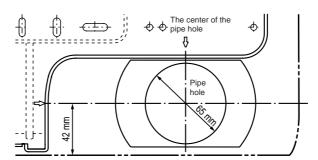
1. After determining the pipe hole position on the installation plate ( ⇒) drill the pipe hole (φ65 mm) at a slight downward slant to the out door side.
