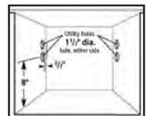
For corner installation, there must be a 1/2" space between the adjacent cabinet doors (i.e. door knobs) and open dishwasher drawer.
