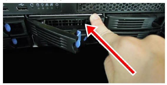
3. Insert the HDD tray into the NVR, and push back the black panel to close it.
