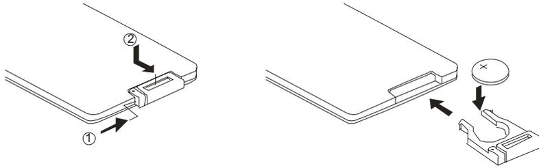
1. Move the small latch to the right and slide out the battery holder.
