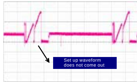
<Fig. 3 When the Set_Down FET is damaged>
