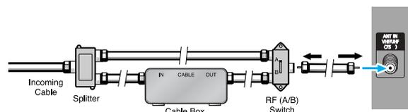
After you've made this connection, set the A/B switch to the "A" position for normal viewing. Set the A/B switch to the "B" position to view scrambled channels. (When you set the A/B switch to "B", you will need to tune your Set-Top Box to the cable box's output channel, which is usually channel 3 or 4.)
