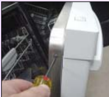
Removing door screws
