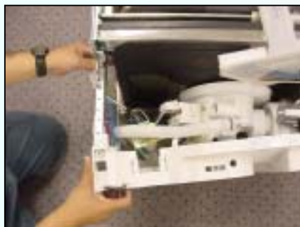
Carefully pull base away from tank & sump
