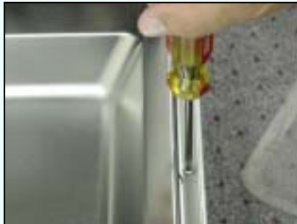
Remove inner door screws
