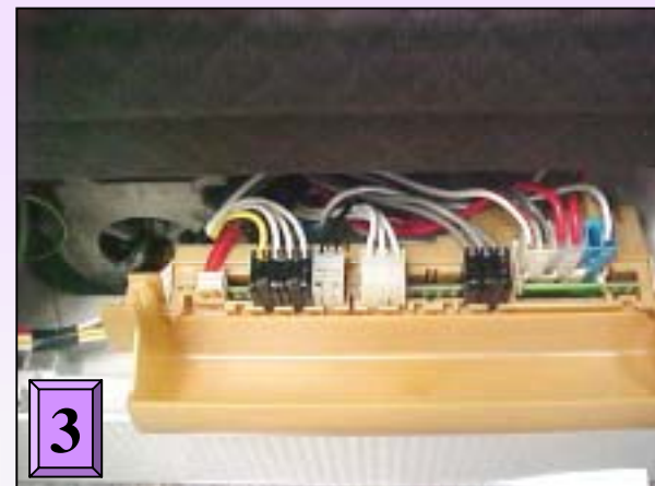
3 Disconnecting module terminals
