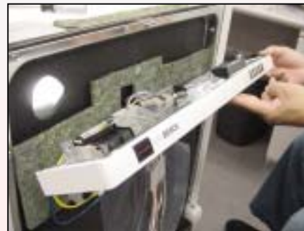
Replace fascia panel
