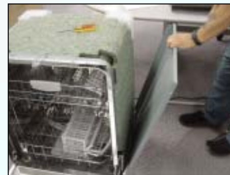
Lift panels up and out
