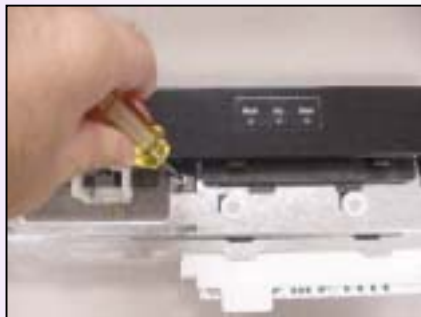
Removing fascia screws
