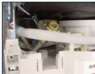
Disconnect water valve from base
