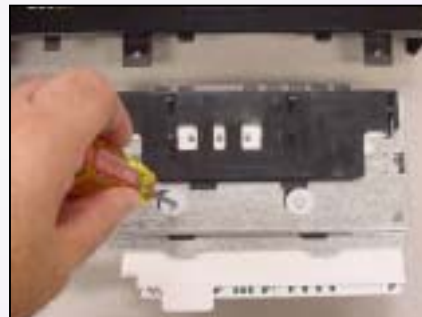
Removing module screws
