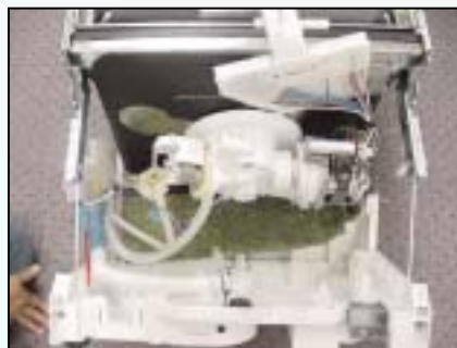
Carefully pull base away from tank & sump
