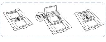
2. Raise the scanner lid (TMA), and place the film holder with the loaded film on the scanner glass bed. Align the arrows so that the holder is flush against the top ruler of the scan bed, with the calibration strip of the holder facing towards the back of the scanner.
