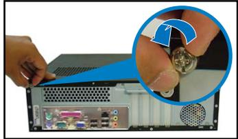
3. Slightly pull the cover toward the rear panel until the cover hooks disengages from the chassis holes.
