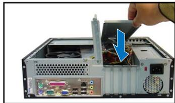
6. Replace the expansion card lock to secure the card to the chassis.
