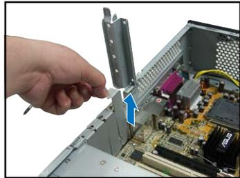
4. Align the card connector with the slot and press firmly until the card is completely seated on the slot.
