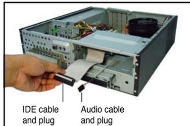
5. Connect the IDE cable to the IDE interface at the back of the drive. Match the red stripe on the cable with Pin 1 on the IDE interface.
