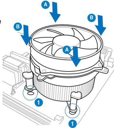
3. When the fan and heatsink assembly is in place, connect the CPU fan cable to the connector on the motherboard.
