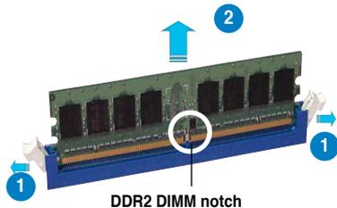
2. Remove the DIMM from the socket.
