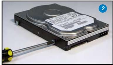
3. Connect one end of the supplied 7-pin SATA cable to the SATA connector at the back of the drive, then connect the other end to a SATA connector on the motherboard. See page 4-7 for the location of the SATA connectors.
