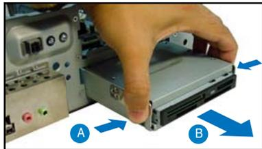
4. Disconnect the USB cable and plug from the card reader assembly, then set the card reader assembly aside.
