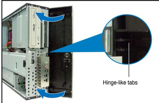
2. Swing the left edge of the front panel inward, then attach the front panel assembly hooks to the chassis until they snap in place.
