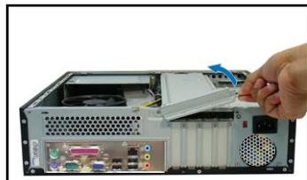
2. Remove the chassis support bracket.
