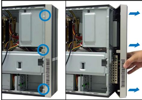
4. Swing the left edge of the front panel assembly outward.
