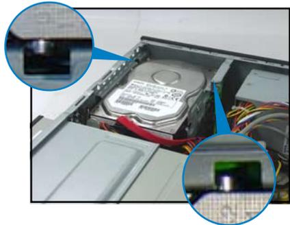
6. When the HDD screws align with the screw rails, push the drive carefully until it is completely flushed on the bay.
