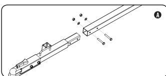
2. Attach the tow bar to the bracket on top of the hydraulic oil tank with two M12x85 bolts and M12 lock nuts. (B)
