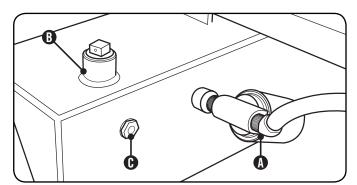
9. Unscrew and remove the tank fill plug, on top of the tank. Using a funnel add approximately 5 gal. (18.9 L) of hydraulic oil to the tank. Wipe up any spilled oil. (B)
