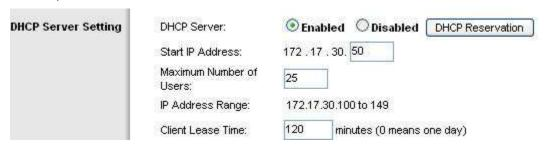
These settings give any PC that connects to this router wirelessly requesting an IP address through DHCP, an address between 172.17.30.50–74. Only 25 clients at a time are able to get an IP address and can only have the IP address for two hours, after which time they must request a new one.
