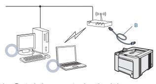
If there is an Ethernet Hub or Router in the same network as the wireless access point of your printer, you can temporarily connect the Hub or Router to the printer using an Ethernet cable (B), this is an easy way to configure the printer. You can then remotely configure the printer from a computer on the network.
