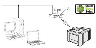
If your wireless access point (A) supports SecureEasySetup™, you do not need to use a computer to configure the printer. The access point (router) and your printer can automatically negotiate using the SecureEasySetup™ procedure. For instructions, see *Using the SecureEasySetup™ software to configure your printer for a wireless network* on page 41.
