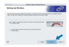
Connect the Brother wireless device to your access point using a network cable and click **Next**. Go to **11**.
