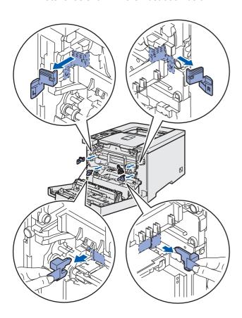
Hold the green handle of the drum unit. Lift the drum unit up and then pull it out until it stops.
