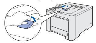
Make sure that the printer power switch is off. Connect the AC power cord to the printer.
