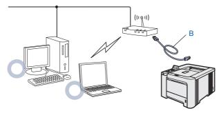
If there is an Ethernet Hub or Router in the same network as the wireless access point of your printer, you can temporarily connect the Hub or Router to the printer using an Ethernet cable (B), this is an easy way to configure the printer. You can then remotely configure the printer from a computer on the network.
