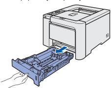
While pressing the green paper-guide release lever (1), slide the paper guides to fit the paper size. Make sure that the guides are firmly in the slots.
