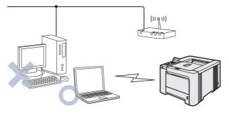
If a computer of yours has wireless capability, you will need to change the wireless settings of the computer to Ad-hoc mode so you can directly connect and configure the printer.
