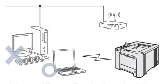
If a computer of yours has wireless capability, you will need to change the wireless settings of the computer to Ad-hoc mode so you can directly connect and configure the printer.
