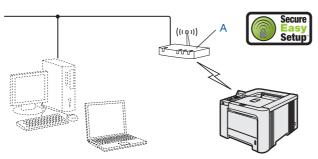
If your wireless access point (A) supports SecureEasySetup™, you do not need to use a computer to configure the printer. The access point (router) and your printer can automatically negotiate using the SecureEasySetup™ procedure. For instructions, see *Using the SecureEasySetup™ software to configure your printer for a wireless network* on page 26.
