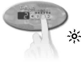
Press and hold **Light** key for five seconds. The display will show a value that represents the filter cycle duration in hours.
