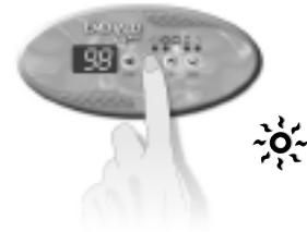
When the desired setting is displayed, press **Light** key again. The filter cycle will start. The "Filter" indicator lights up when a filter cycle is on.
