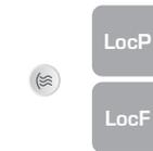
When control pad is locked, all automatic functions of the system run as usual. If a key is pressed down, a “LocP” or “LocF” message will be displayed for 1 second. To unlock the keypad, simply press and hold Pump 1 key again for five seconds.
