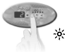
Press and hold **Light** key for 5 seconds. The display will show a value that represents the filter cycle duration in hours.
