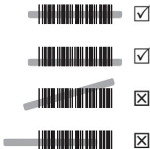
To scan a barcode, make sure the aiming beam crosses every bar and space of the barcode.
