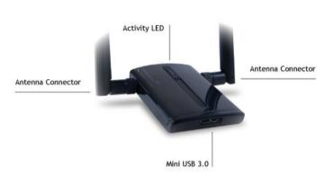
Mini USB 3.0: The included USB 3.0 cable attaches to the Mini USB connector on the Adapter. The other end connects to available USB ports on your PC. For maximum speed, a USB 3.0 port is required. The adapter is backwards compatible with USB 1.0 and 2.0 but will function at lower speeds. Do not attach the cable until after you have installed the software.
