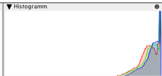
Fig. 43: In this example, the right end of the Shading histogram curve is clipped. Shading images with histograms that are "squeezed" against the left or the right side of the scale lead to inaccurate Shading corrections.
