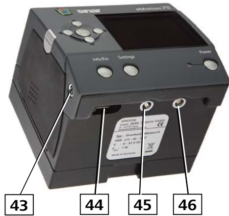
Fig. 20: Connector sockets on Sinarback eMotion 75/54
