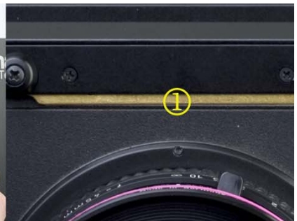
Fig. 17: The lens latching slider
