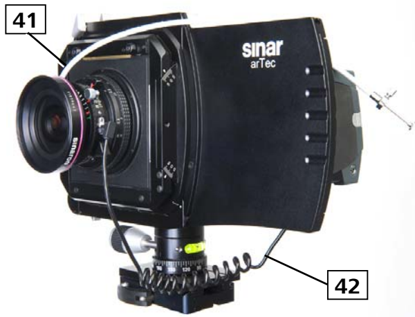
Fig. 19: Sinar arTec with attached release cables
