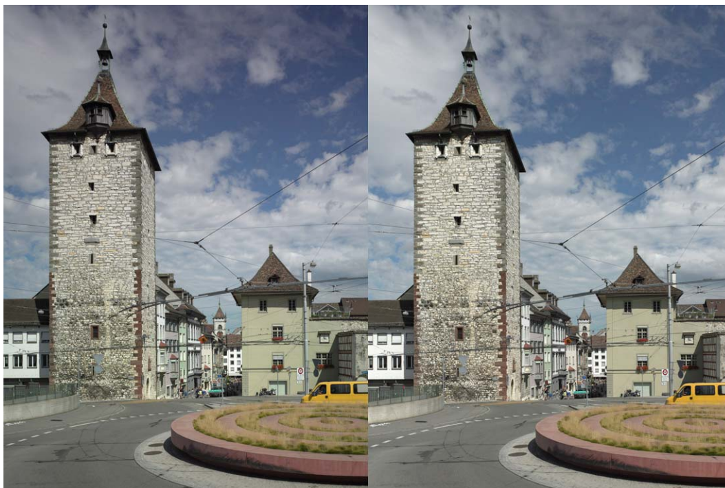
Fig. 47: Left: Noticeable loss of brightness at the top of the tower and in the white cloud above it. Right: Homogeneous lighting across the entire image field, thanks to the Shading correction.
