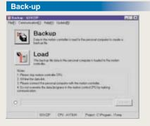
• Back-up of motion controller programs, parameters and internal information in a batch as a file
