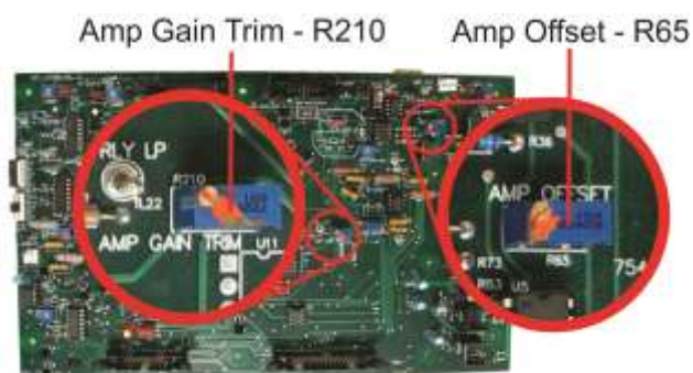
Figure 4.10 – Main Board Balancing Control Locations
