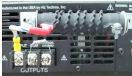
Figure 4.3 – 7224 Ballast Resistor Connected to Output Terminal
