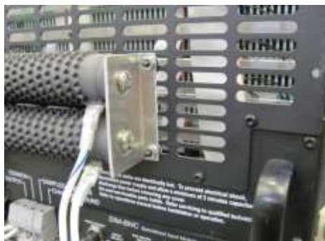
Figure 4.2 – 7796 Ballast Resistor Mounting
