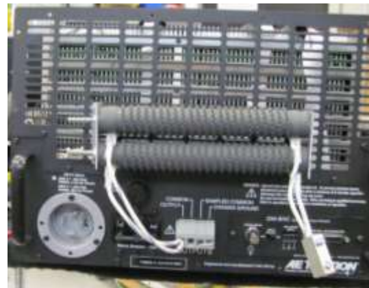
Figure 4.4 – 7796 Ballast Resistors Connected to Output Terminal (Note: Kits for 7548 amplifiers contain one ballast resistor)
