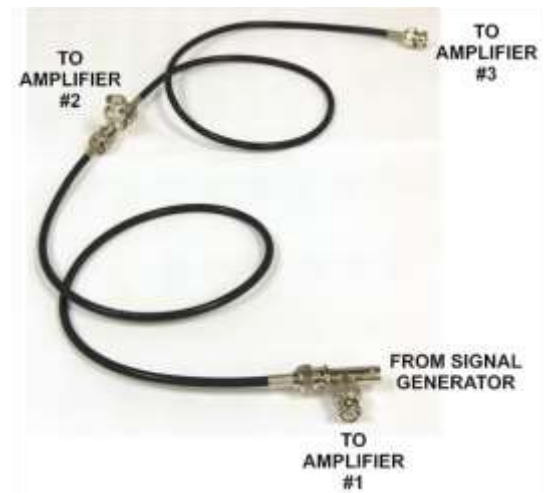
Figure 4.13 – Optional BNC Parallel Input Wiring (Three in Parallel shown)
