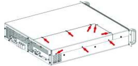
Figure 3.3 – 7224 Amplifier Access Panel Screw Locations
