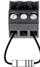
Figure 3.12 – Terminating the Amplifier Input
