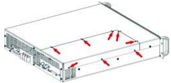
Figure E-1 – 7224 Access Panel Screw Locations
