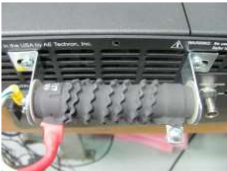
Figure 4.1 – 7224 Ballast Resistor Mounting
