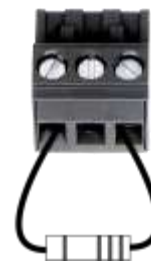
Figure 3.7 – Terminating the Amplifier Input
