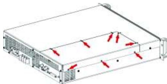
Figure 4.5 – Access Panel Screw Locations
