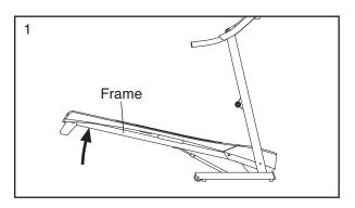
2. Hold the treadmill firmly with your right hand as shown. Pull the latch knob to the left and hold it. Raise the frame until the catch is past the latch pin. Then, slowly release the latch knob; **make sure that the catch is resting against the latch pin.**
