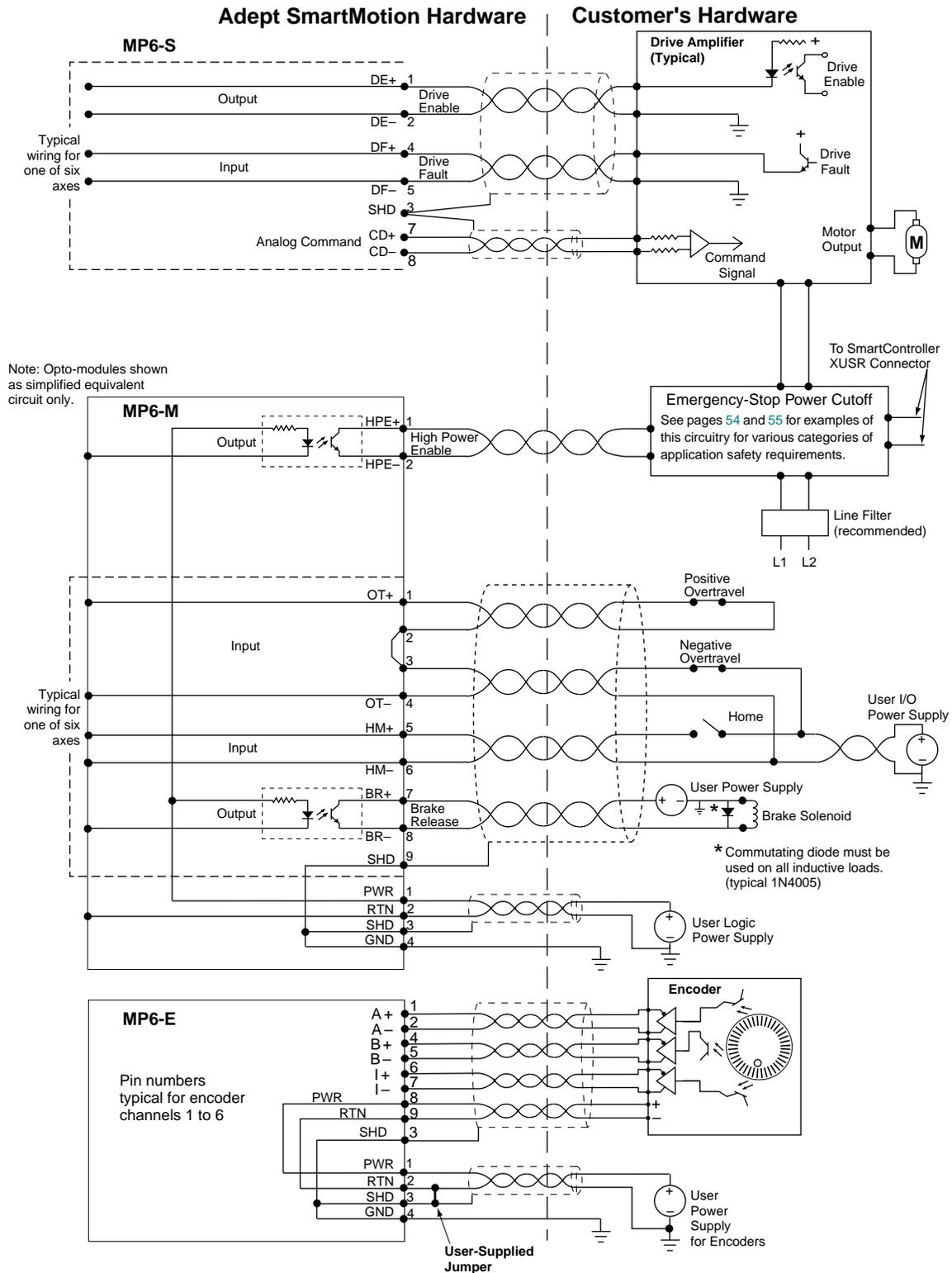
Figure 2-9. Typical System Wiring for One Axis of Motion
