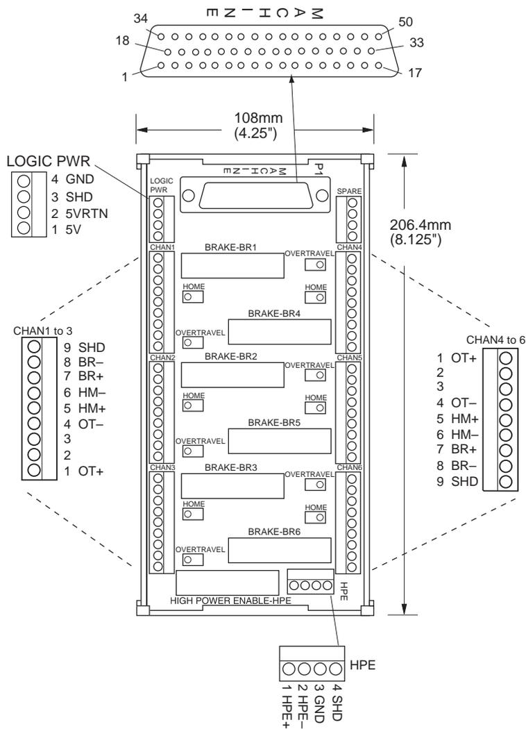
Figure 2-8. MP6-M Panel - Layout and Dimensions
