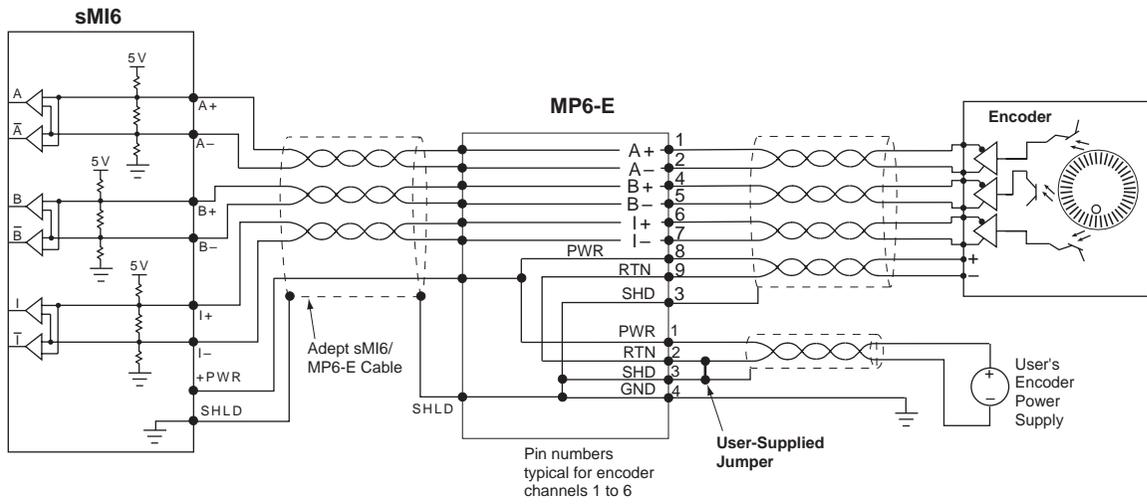
Figure 2-10. Encoder Input Circuitry
