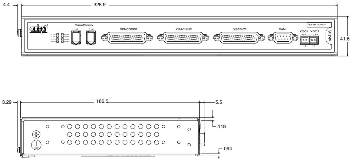
Figure 4-1. Dimensions for sMI6 Module
