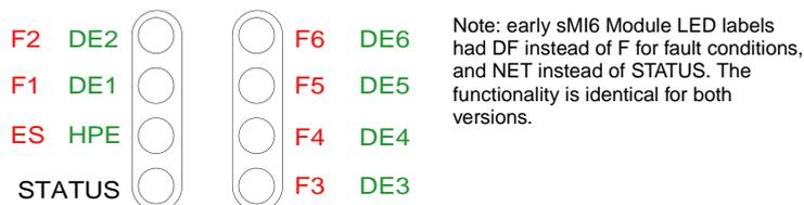
**Figure 2-1. Close-up of sMI6 LED Labels**
