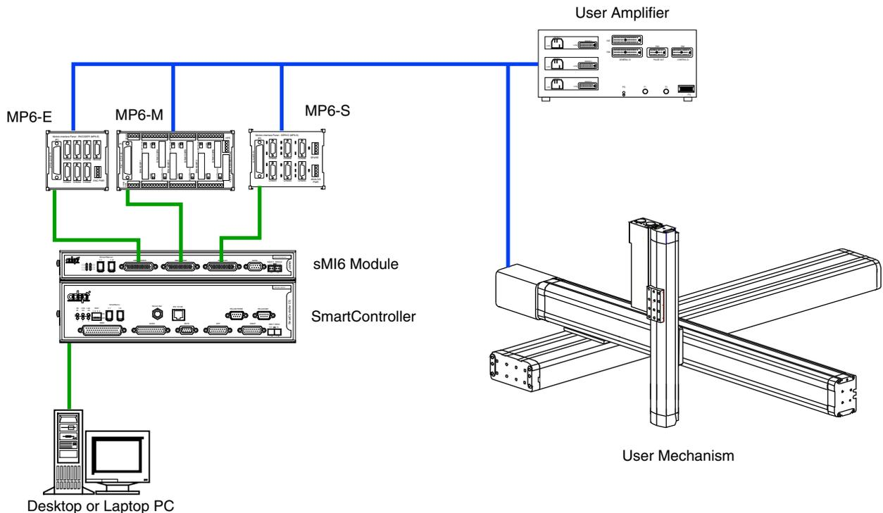
Figure 3-1. SmartMotion System Installed to Control a User Mechanism
