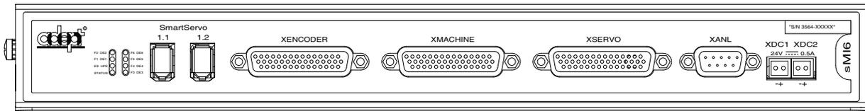
Figure 2-2. Adept sMI6 Module Front Panel
