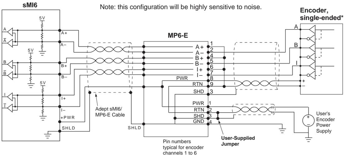
\*Note: this configuration leads to inversion of the encoder channel signals. Remember this when using the SPEC program to specify the Zero-Index configuration.
