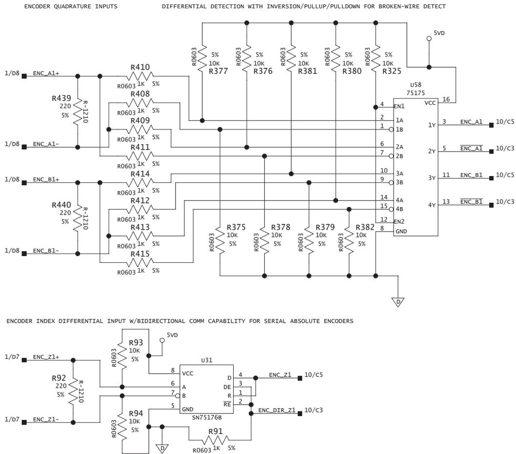
Figure 2-11. Encoder Input Schematic
