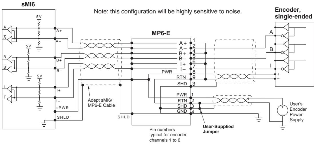
Figure 2-12. Single-Ended Encoder Wiring Using Inverted Outputs
