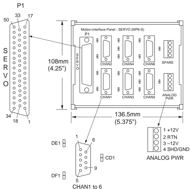
Figure 2-6. MP6-S Panel - Layout and Dimensions
