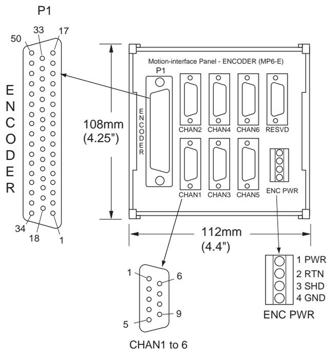
Figure 2-7. MP6-E Panel - Layout and Dimensions
