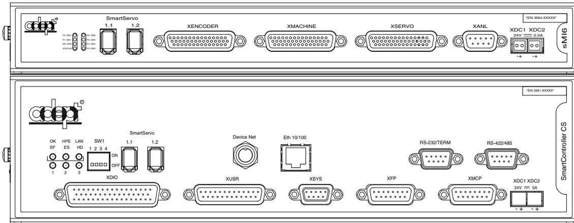
**Adept SmartController CS with sMI6 Motion Interface Module**
