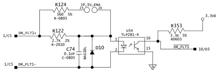
**Figure 4-5. Typical Input Circuit in sMI6**
