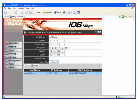
**Host Name:** Type the host name in the text box. The host name is required by some ISPs. The default host name is "AP-Router."
