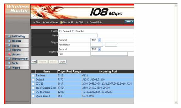
**Enable:** Click to enable or disable the application profile. When enabled, users will be able to connect to the application via the router WAN connection. Click Disabled on a profile to prevent users from accessing the application on the WAN.
