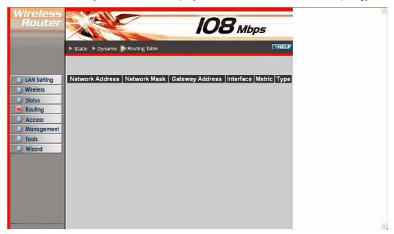
**Network Address:** Displays the network IP address of the connected node. **Network Mask:** Displays the network (subnet) mask of the connected node. **Gateway Address:** Displays the gateway address of the connected node. **Interface:** Displays whether the node is connected via a WAN or LAN.
