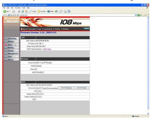
**Firmware Version:** Displays the latest build of the router firmware interface. After updating the firmware in Tools - Firmware, check this to ensure that your firmware was successfully updated.
