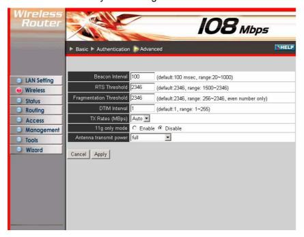
**Beacon Interval:** Type the beacon interval in the text box. You can specify a value from 1 to 1000. The default beacon interval is 100.
