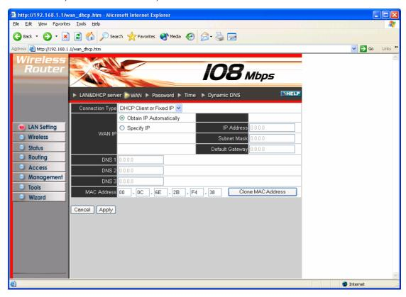
**Connection Type:** Select the connection type, either DHCP client, Fixed IP or PPPoE from the drop-down list.
