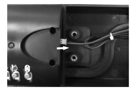
3. Pull out the pin socket as photo shown.
