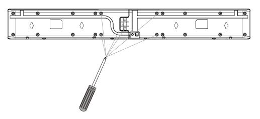
1. At the rear cabinet, loosen screws (6 pcs is necessary) as photo shown using a Philips screwdriver.
