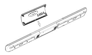
3. Install the front panel as photo shown
