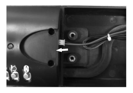
2. Insert the pin socket as photo shown
