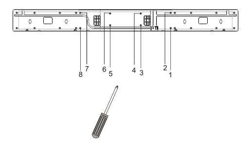
4. Finally, fix it with 8 screws as photo shown
