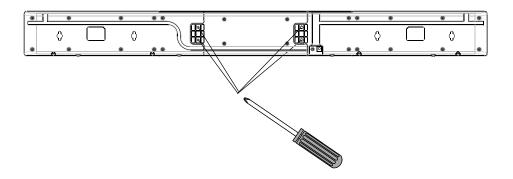
1. Screws (4 pcs) the extender with left and right bars as photo shown.
