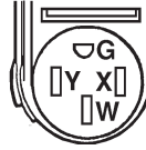
4-wire wall receptacle (14-50R)
