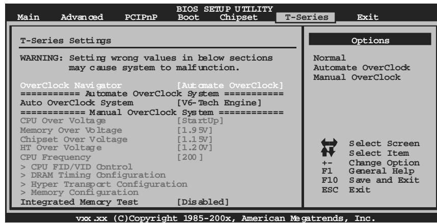
The Overclock Navigator provides 3 different engines helping you to overclock your system. These engines will boost your system performance to different level.
