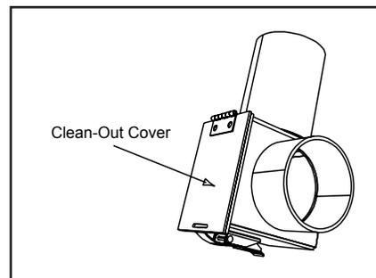
Figure 18.4 - Rear to Top Vent Adapter - 90°
