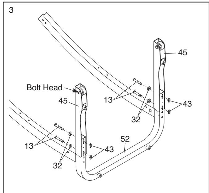
4. Position the Base (52) as close to the front of the treadmill as possible, as shown.
