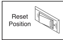
**IMPORTANT:** The console features a display demo mode, designed to be used if the treadmill is displayed in a store. If the displays light as soon as you plug in the power cord and switch the reset/off circuit breaker to the reset position, the demo mode is turned on. To turn off the demo mode, hold down the Stop button for a few seconds. If the displays remain lit, see THE INFORMATION MODE on page 19 to turn off the demo mode.
