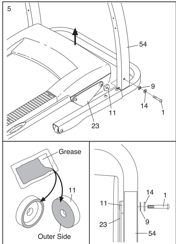
6. **See the inset drawing in step 5.** Identify the outer side of the remaining Frame Spacer (11).
