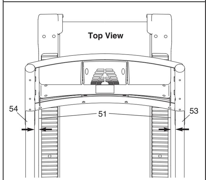
13. Attach the Left Crosswalk Arm (117) and a Plastic Spacer (119) to the Left Upright (53) with two 1/4" Flat Washers (114) and two 1/4" x 3" Bolts (111). **Make sure that the Left Crosswalk Arm is on the indicated side of the Console (91).**
