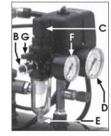
Before connecting your airline to the compressor, allow it to run for 10 - 15 seconds, with the air outlet tap, (G, Fig. 2) completely open to permit a good distribution of the lubricating oil.
