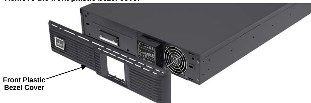
Figure 7 Remove the front plastic bezel cover
