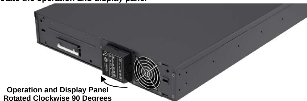
Figure 8 Rotate the operation and display panel
