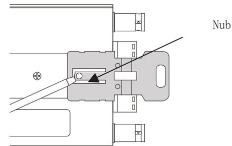
2. While lifting the nub, slide the bracket out in the direction of the arrow as shown below:
