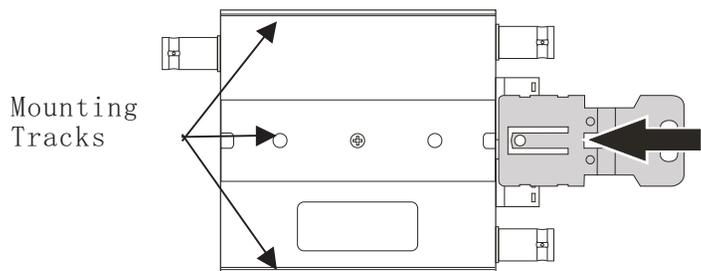
2. Slide the bracket in the direction of the arrow until the white nub clicks into place as shown below:
