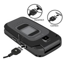
Note: The previous illustration displays the incorrect method for connecting the charger. If attempted, damage to the accessory port will occur therefore voiding the phone's warranty.
