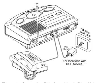
Figure 4 – Connecting Telephone Line to Base Unit
