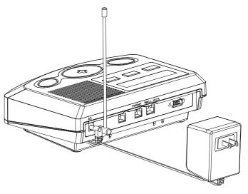
Figure 5b – Inserting Plug into Base Unit
