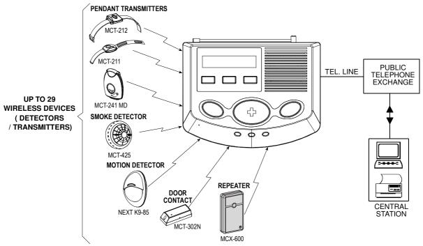
Figure 2 - System Configuration
