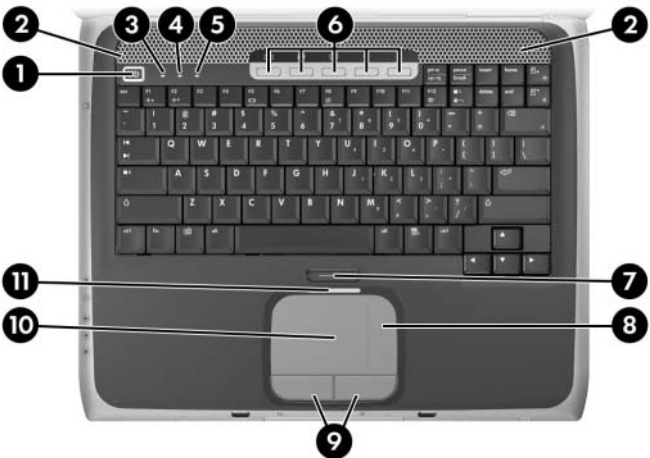
Top Components - HP Pavilion ze4900
