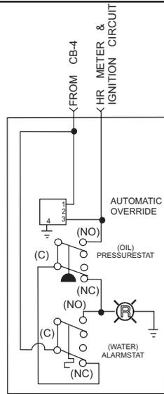
**NOTE:** ALARMSTAT AND PRESSURESTAT ARE SHOWN WITH ENGINE OFF.
