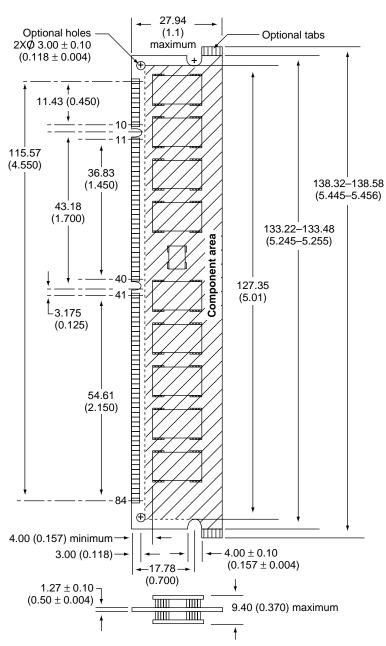
Note: Dimensions are in millimeters (inches).
