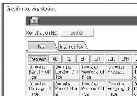
You can change the display to the fax destination, Internet fax destination, and IP-Fax destination using the key on the left side of the display.
