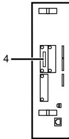
When the wireless LAN board (optional) is installed.
