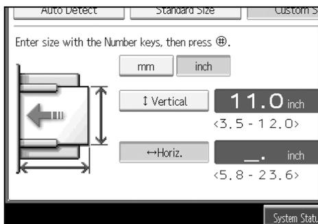
Specify a horizontal size from 148 mm (5.9") to 600 mm (23.7"). You cannot enter a size smaller than 148 mm or larger than 600 mm.
