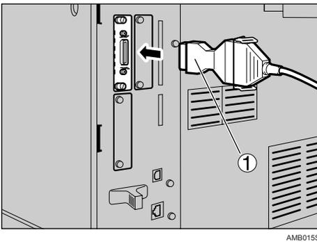
Use the conversion connector (1) supplied with the IEEE 1284 interface board.
