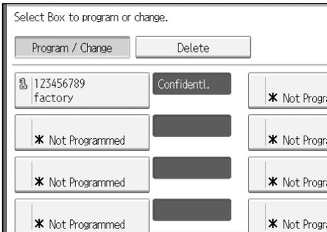
To change a box already programmed, press it, and then proceed to step **3**. If a password is programmed, enter the password, press **[OK]**, and then proceed to step **3**.
