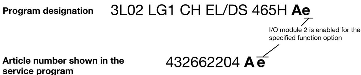
If the machine subsequently fitted with I/O module 2, the module will acquire the function option as specified by the second letter once the new I/O module has been addressed.
