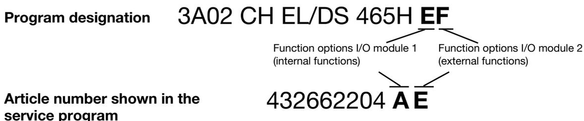
If the second letter (I/O module 2) appears in lower case, it means that the machine is not fitted with I/O module 2 but the downloaded parameter software is I/O module 2 enabled.
