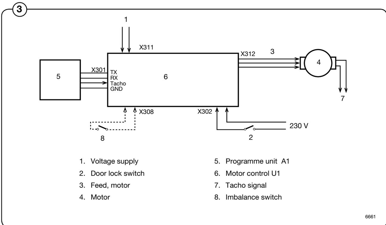
The motor control is also able to deliver the various instantaneous and output values during constant speed, acceleration and retardation. These values are used to calculate the weight of the loaded laundry and to detect any load imbalances. A separate imbalance switch can also be connected to the motor control.
