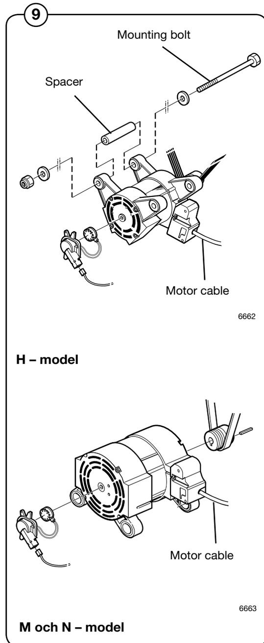
3. Connect the new motor to the cable and use straps to secure the cable.
