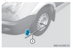
Loosen the wheel nuts or wheel bolts on the wheel to be changed by about one turn using extended lug wrench ①. Do not unscrew the wheel bolts or wheel nuts completely.
