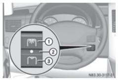
Central control switch for the rear interior lighting
