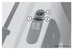
Button and switch for mirror adjustment
