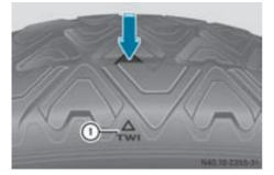
Bar marking 1 for tread wear is integrated into the tire tread.
