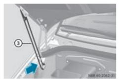
Swing the hood upwards until support strut
