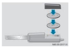
▶ Remove old batteries from the battery tray.
