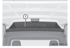
On vehicles with a partition, stowage space (1) can be loaded from the cargo compartment.
