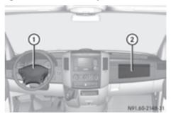
Driver's front air bag ① deploys in front of the steering wheel; co-driver's front air bag ② deploys in front of and above the glove box. They are deployed:
