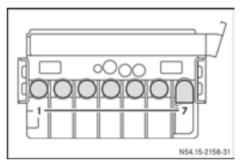
Prefuse box in the battery compartment in the driver's footwell F59
