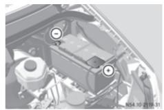
Additional battery in the engine compartment
