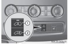
When the automatic locking when driving function is activated, there is a risk of being locked out if the vehicle is being pushed or towed.
