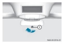
► Anti-glare mode: push anti-glare lever ① in the direction of the arrow.
