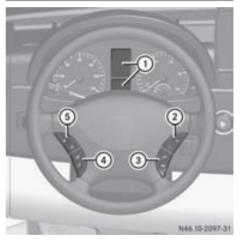
You can control the display and the settings in the on-board computer with the buttons on the steering wheel.
