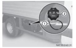
DEF tank on the right-hand side of the vehicle (example: Chassis Cab)
