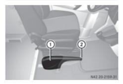
Only apply the parking brake when the vehicle is stationary.
