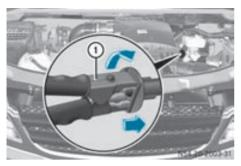
Jump-starting connection point left of the air filter
