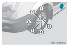
Tightening torque pattern ①-⑥ Wheel bolts or wheel nuts
