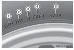
The TIN is a unique identification number. The TIN enables the tire manufacturers to inform purchasers of recalls and other safetyrelevant matters. It makes it possible for the purchaser to easily identify the affected tires. The TIN is made up of manufacturer identification code (2), tire size (3), tire type code (4) and date of manufacture (5).
