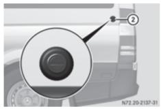
With the rear door opened to an angle of 270°, push it against magnetic door retainer (2) on the side wall.
