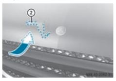
Push hood catch release handle (2) upwards.
