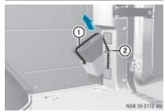
Wheel chock in the load/passenger compartment
