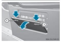
The fuse box is located on the outside of the base of the driver's seat.
