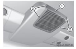
Air filter in the roof in the rear compartment
