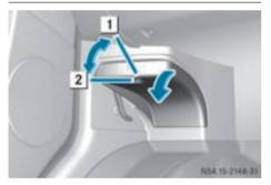
The fuse box is located in the footwell on the lefthand side of the vehicle.
