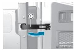
• Vehicles with 270° pivoting rear doors: If you prefer to keep door retainer ① out of the loading area when loading the vehicle, you can swivel it 180° against the spring force and onto the door and engage it. The door retainer remains in this position and will not swivel back to its original position.
